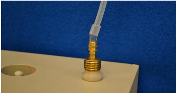
Figure 5. VAPOR PIN® sample connection
