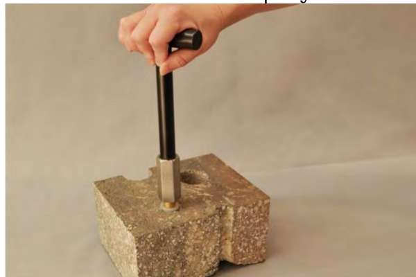
Figure 7. Removing the VAPOR PIN®
